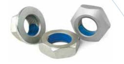
This metal-to-metal contact provides a positive resistance to vibration and loosening. Since nylon has great memory characteristics, this locking element is reusable. NylokHD® Patch can be applied to nuts of any style or plating. A wide range of nut sizes can be processed.
