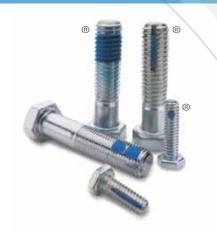
When the pellet & strip are engaged it creates a wedge between the fastener and mating part compressing the nylon and creating metal to metal contact opposite the element. This metal to metal contact results in a positive resistance to vibration and loosening. Since nylon has great memory characteristics, this locking element can be reused several times.
