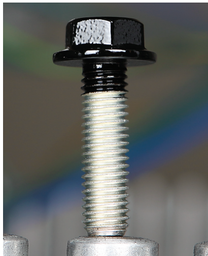
CONTROL: ELECTROPLATE ZN FINISH
