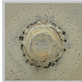
CONTROL: ELECTROPLATE ZN FINISH
