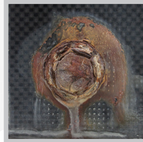
CONTROL: ELECTROPLATE ZN FINISH
