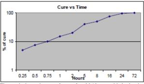
The graph shows the rate of cure of an M-10 nut and bolt plated with various finishes. The breakaway strength was determined using industrial procedures.
