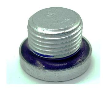
M18 Fastener Used for All Testing Zinklad 250 + TNT-15
